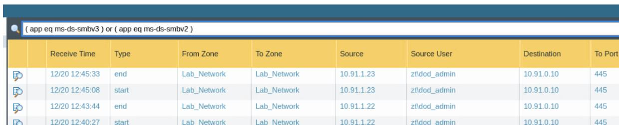
The screenshot shows the Palo Alto Networks interface with the filter **( app eq ms-ds-smbv3 ) or ( app eq ms-ds-smbv2 )** applied. The traffic logs table is displayed with the following data:
